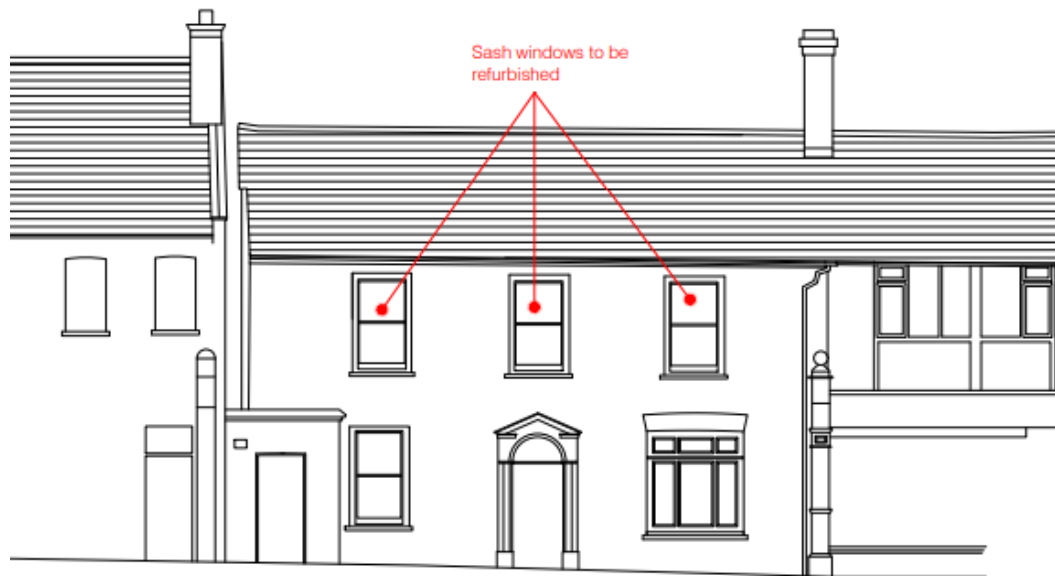
SOUTH EAST ELEVATION (FRONT)
